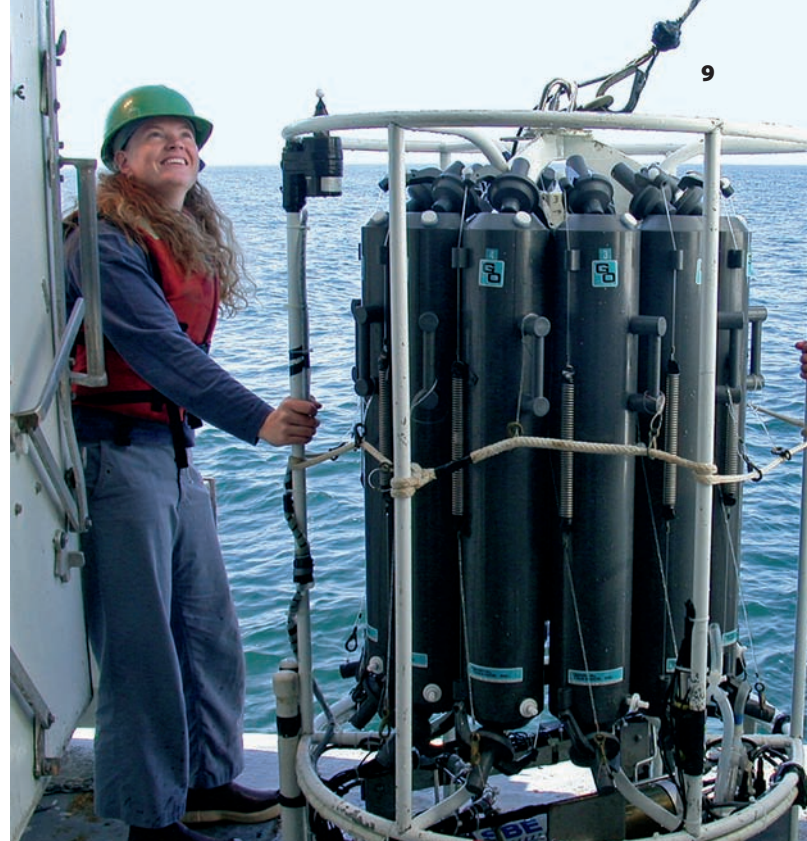
Figure 1.5 This instrument consists of numerous bottles that are submerged to collect water samples from the ocean.
